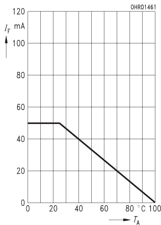
Figure 4. Maximum Permissible Forward Current,  $I_F = f(T_A)$ ,  $R_{\text{thJA}} = 450 \text{ K/W}$
