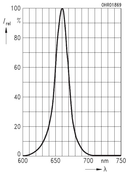
Figure 1. Relative Spectral Emission  $I_{\text{rel}} = f(\lambda)$
