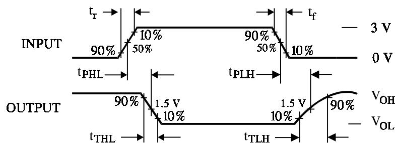
Figure 1. Switching Waveforms
