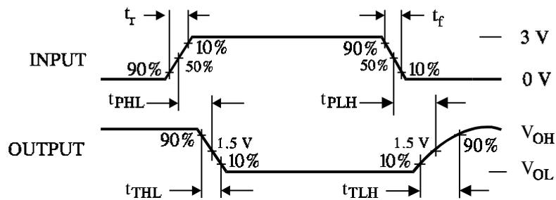
Figure 1. Switching Waveforms
