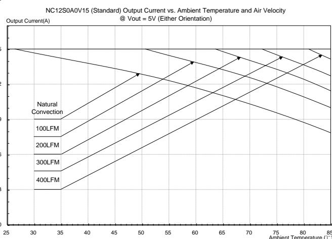
**Figure 34:** Output current vs. ambient temperature and air velocity @  $V_{out}=5V$  (Either Orientation)
