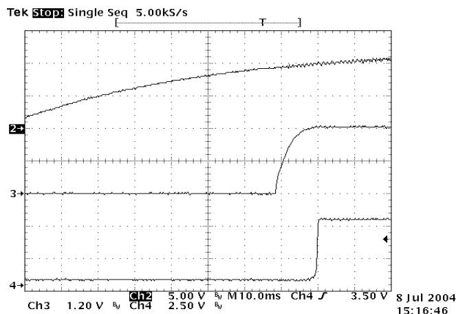
**Figure 15:** Turn on delay time at 12Vin, 2.5V/15A out
