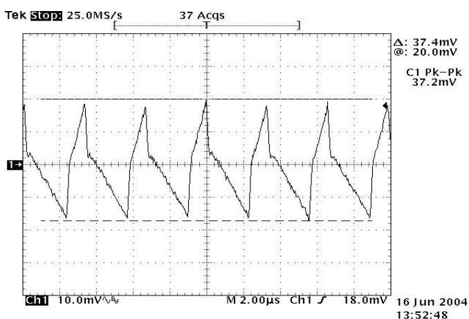
Figure 11: Output ripple & noise at 12Vin, 3.3V/15A out
