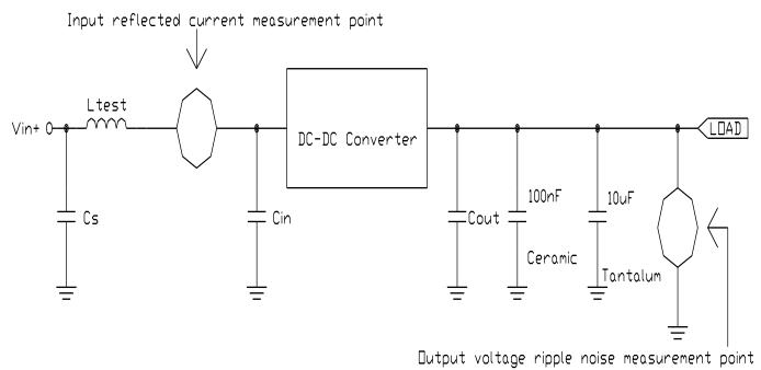
$C_s = 270\mu F * 1$ ,  $L_{test} = 1.4\mu H$ ,  $C_{in} = 270\mu F * 1$ ,  $C_{out} = 680\mu F * 1$
