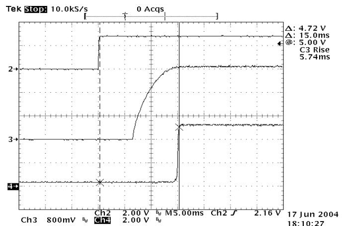
**Figure 16:** Turn on delay time at Remote On/Off, 2.5V/15A out
