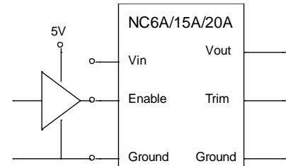
Figure 25: Enable input drive circuit using logic gate.
