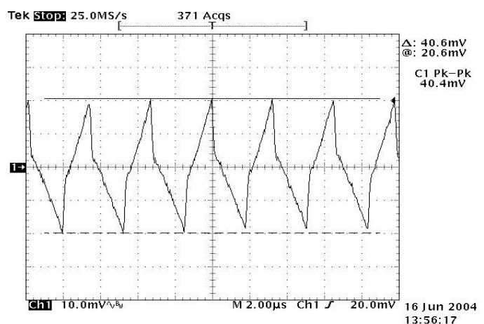
Figure 12: Output ripple & noise at 12Vin, 5.0V/15A out
