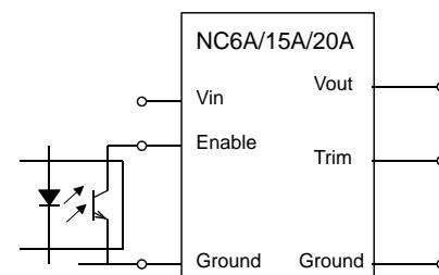
Figure 26: Enable input drive circuit example with isolation.
