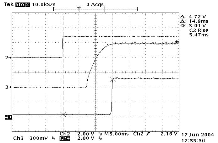
**Figure 14:** Turn on delay time Remote On/Off, 0.9V/15A out
