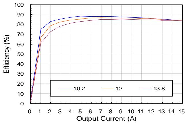
**Figure 3:** Converter efficiency vs. output current
