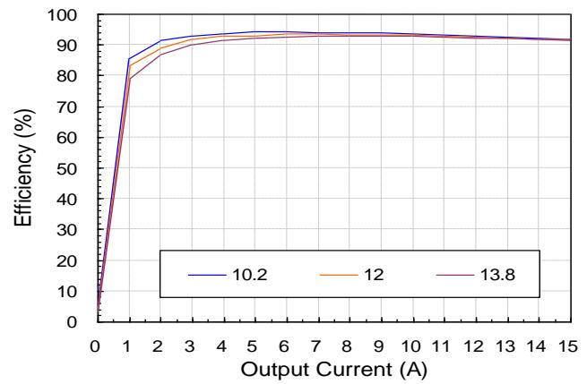
**Figure 6:** Converter efficiency vs. output current
