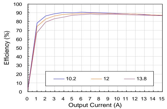
**Figure 4:** Converter efficiency vs. output current
