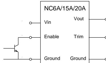
Figure 24: Enable Input drive circuit for NC series
