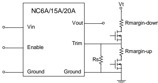
**Figure 30:** Circuit configuration for output voltage margining
