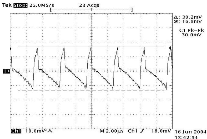
Figure 9: Output ripple & noise at 12Vin, 1.8V/15A out
