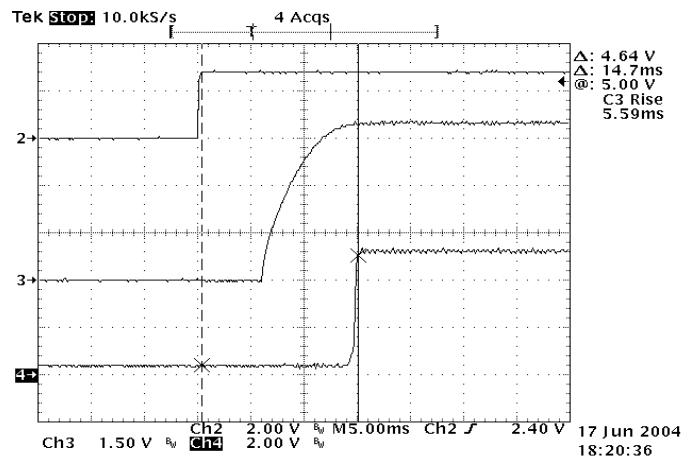
**Figure 18:** Turn on delay time at Remote On/Off, 5.0V/15A out
