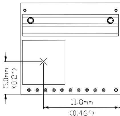
**Figure 39:** Temperature measurement location
