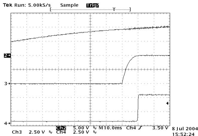
**Figure 17:** Turn on delay time at 12Vin, 5.0V/15A out
