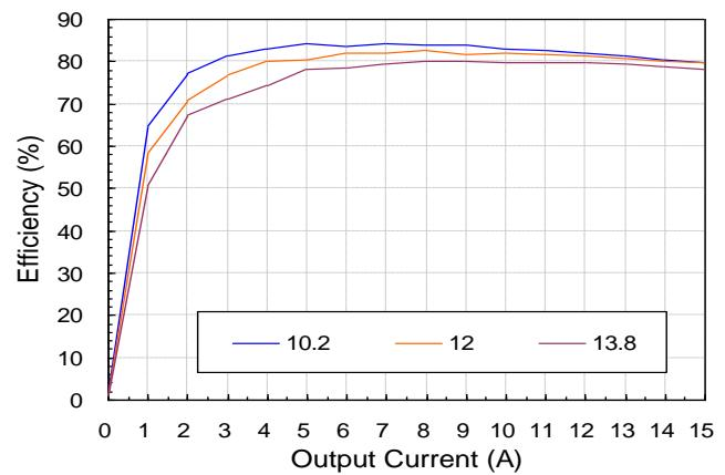
**Figure 2:** Converter efficiency vs. output current
