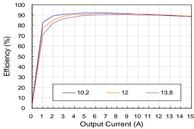
**Figure 5:** Converter efficiency vs. output current
