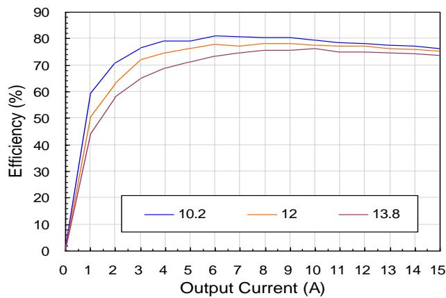
**Figure 1:** Converter efficiency vs. output current
