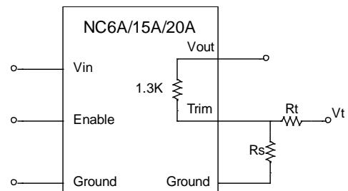
**Figure 29:** Output voltage trim with voltage source
