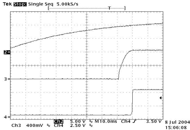
**Figure 13:** Turn on delay time at 12Vin, 0.9V/15A out
