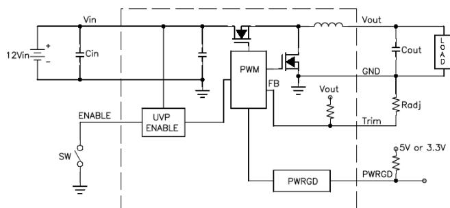
Figure 23: Block Diagram
