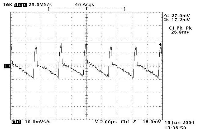
Figure 8: Output ripple & noise at 12Vin, 1.2V/15A out
