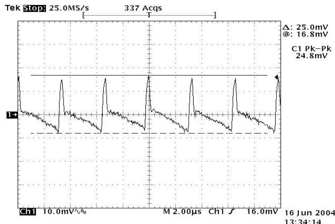
Figure 7: Output ripple & noise at 12Vin, 0.9V/15A out
