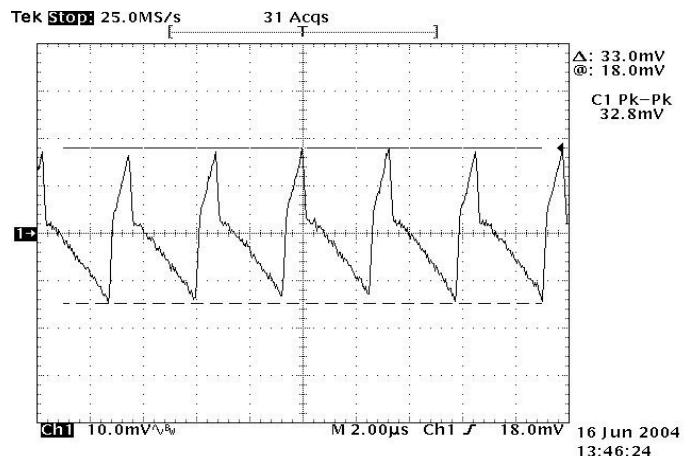
Figure 10: Output ripple & noise at 12Vin, 2.5V/15A out
