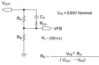
**Figure 6:** V<sub>OUT</sub> Resistor Divider & Compensation Components. RA equation is only valid for Best Performance option. For Small Solution Size option, see Table 5.
