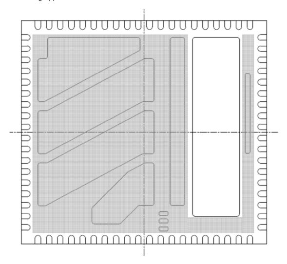
Figure 10: Lead-Frame exposed metal (Bottom View)
