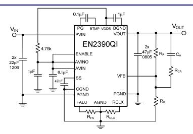
Figure 1. Simplified Applications Circuit (Footprint Optimized)
