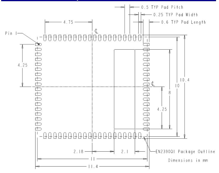
Figure 11: EN2390QI PCB Footprint (Top View)
