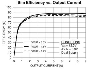
Figure 7: Efficiency vs. Output Current
