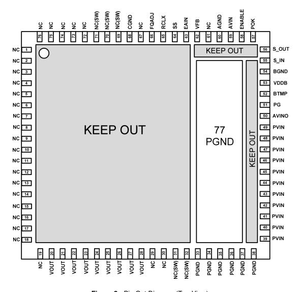
Figure 3: Pin Out Diagram (Top View)
