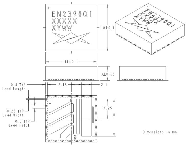
Figure 12: EN2390QI Package Dimensions (Bottom View)
