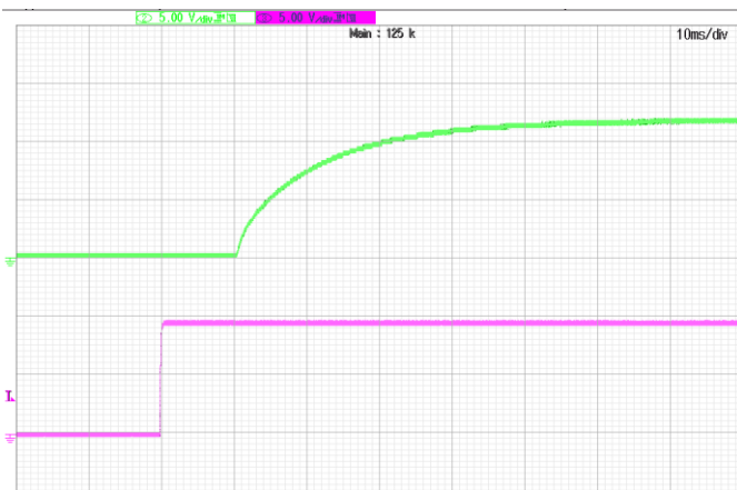
Turn-on transient at full load current (10ms/div). Top Trace: Vout; 5V/div; Bottom Trace: ON/OFF input: 5V/div.
