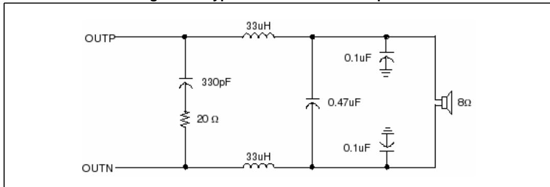
**Figure 26. Typical LC filter for a 4 Ω speaker**
