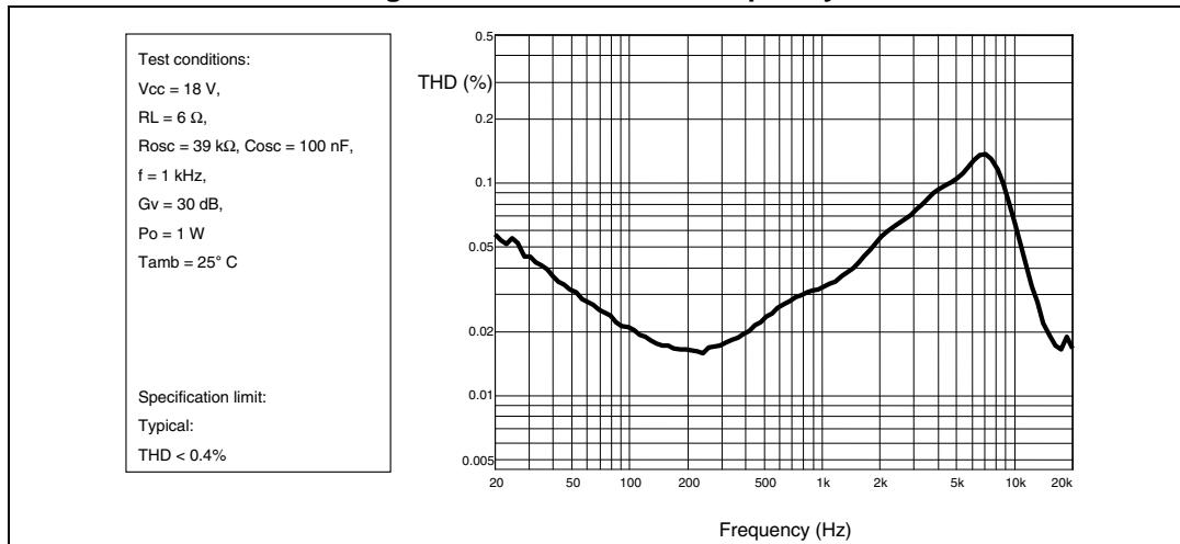
**Figure 7. Frequency response**
