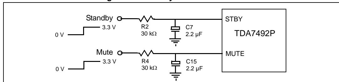
**Figure 22. Turn-on/off sequence for minimizing speaker “pop”**
