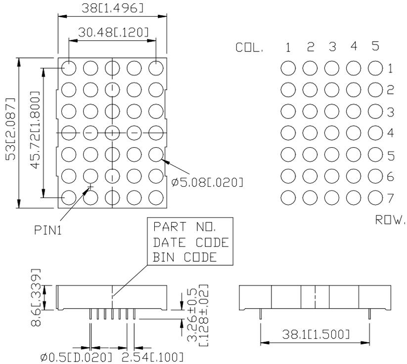
NOTES: All dimensions are in millimeters. Tolerance is  $\pm 0.25$  mm (0.01") unless otherwise noted.
