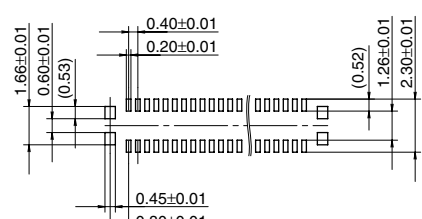
Recommended metal mask pattern Metal mask thickness: When 120µm (Terminal opening ratio: 70%) (Metal-part opening ratio: 100%)
