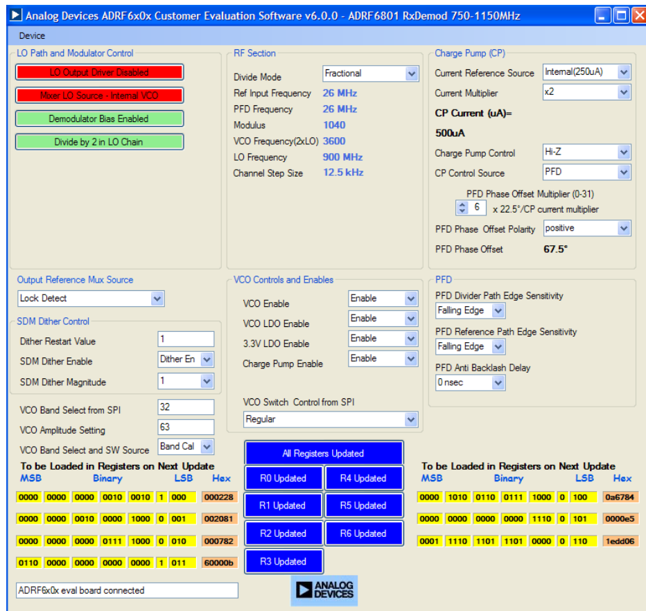
Figure 46. Evaluation Board Software Main Window
