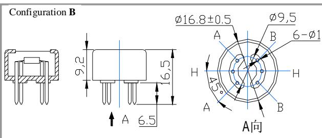
Structure and configuration of MQ-3 gas sensor is shown as Fig. 1 (Configuration A or B), sensor composed by micro  $\text{Al}_2\text{O}_3$  ceramic tube, Tin Dioxide ( $\text{SnO}_2$ ) sensitive layer, measuring electrode and heater are fixed into a crust made by plastic and stainless steel net. The heater provides necessary work conditions for work of sensitive components. The enveloped MQ-3 have 6 pin ,4 of them are used to fetch signals, and other 2 are used for providing heating current.
