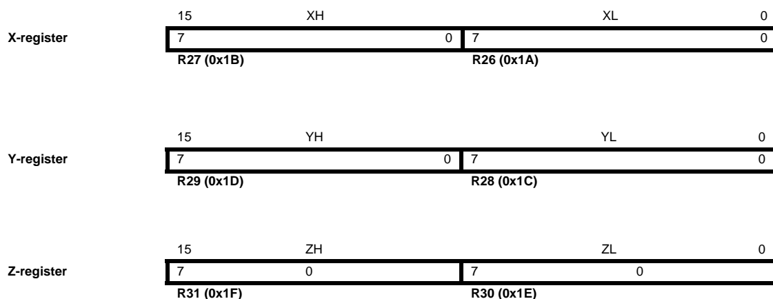
Figure 4-3. The X-, Y-, and Z-registers
