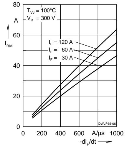
Fig. 3 Peak reverse current  $I_{RM}$  versus  $-di_F/dt$
