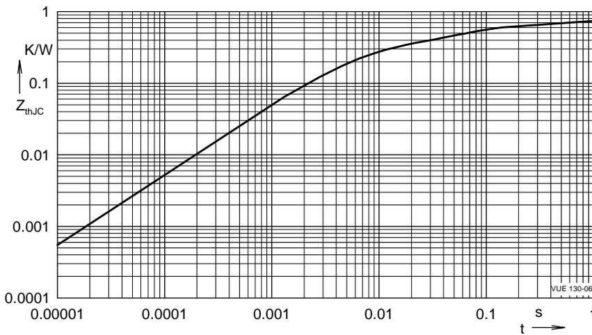
Fig. 7 Typical transient thermal resistance junction to case
