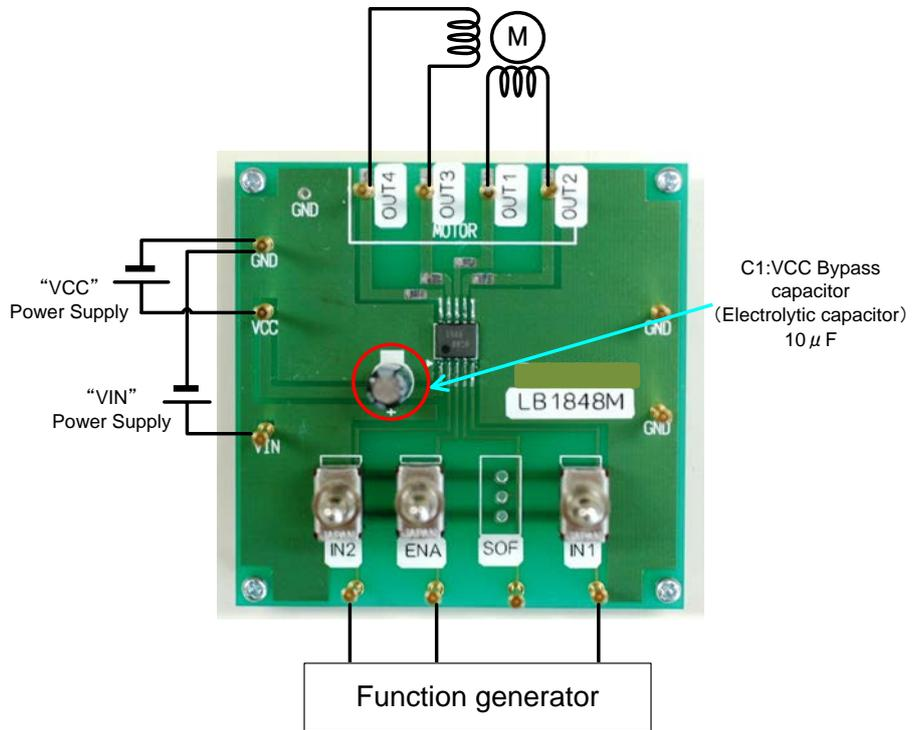
(Circuit diagram of the evaluation board)
