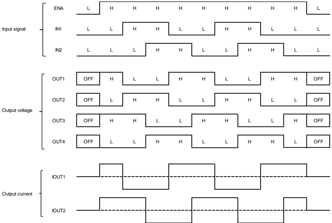
•Stepper motor driving waveform example
