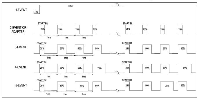
Figure 2. MEC Waveforms in Different Scenarios
