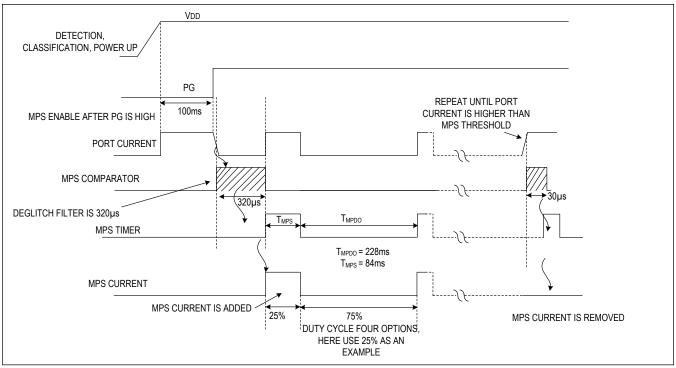
Figure 3. Intelligent MPS Behavior
