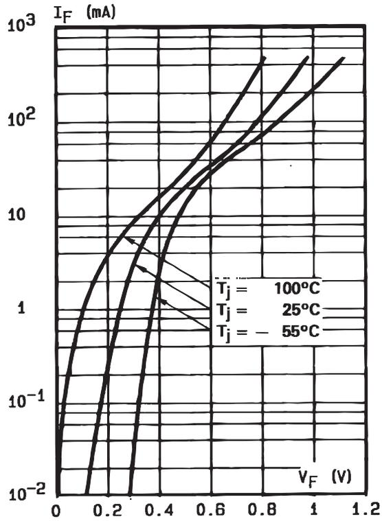
**Fig. 2:** Forward current versus forward voltage (typical values).
