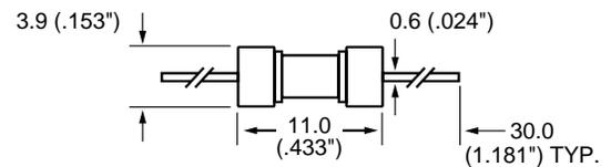
Axial Lead Material: Solder coated copper.
