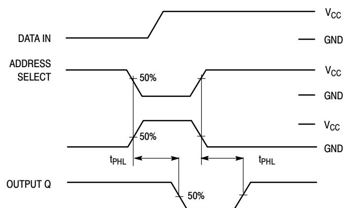
Figure 7. Switching Waveform
