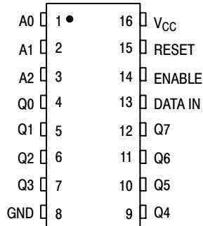
Figure 2. Pin Assignment
