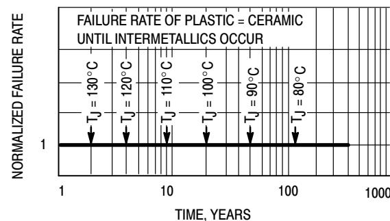
Figure 5. Failure Rate vs. Time Junction Temperature
