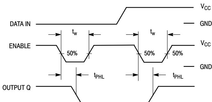
Figure 8. Switching Waveform
