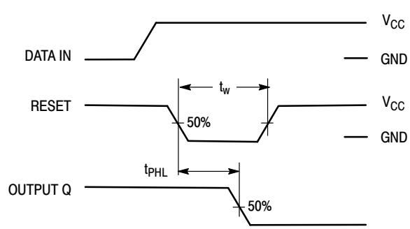
Figure 9. Switching Waveform
