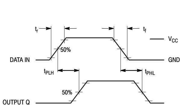
Figure 6. Switching Waveform
