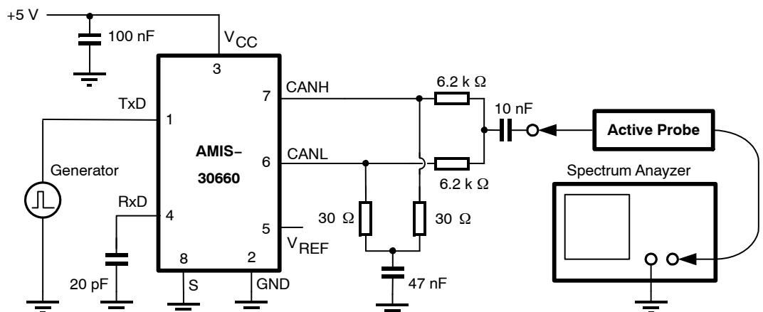
**Figure 7. Basic Test Set-up for Electromagnetic Measurement**
