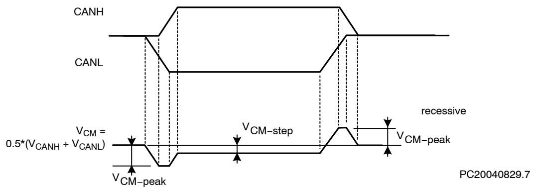
**Figure 8. Common-Mode Voltage Peaks (see Measurement Setup)**
