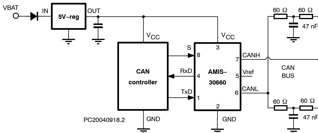
**Figure 2. Application Diagram**
