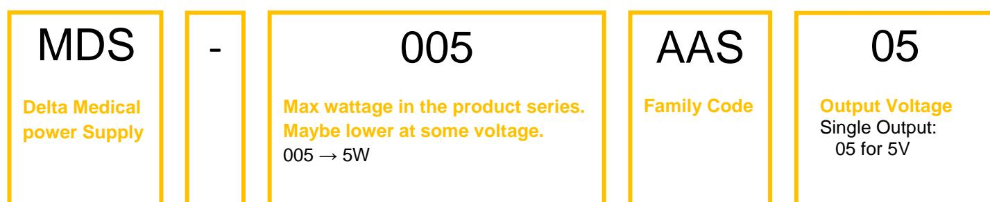
**MDS Medical AC-DC Wall Mount Adapter****5Volt, 5Watt / MDS-005AAS05 B****Specifications****Input Ratings / Characteristics**
