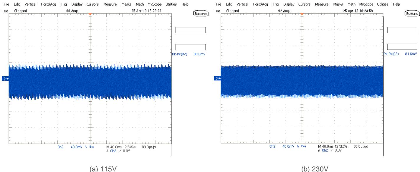
Fig. 2 Ripple &amp; Noise example, 20MHz BW
