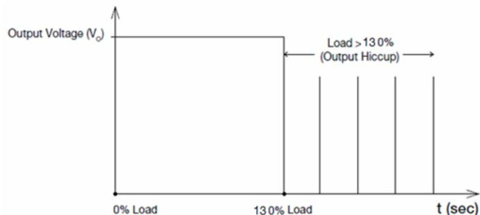
Additionally, if the  $I_o$  is  $<130\%$  but  $>110\%$  for a prolong period of time (depending on the load), the Over Temperature Protection (OTP) will be activated due to high temperature on critical components. The power supply will then go into hiccup mode until the fault is removed; and, the input voltage is removed, then reapplied.
