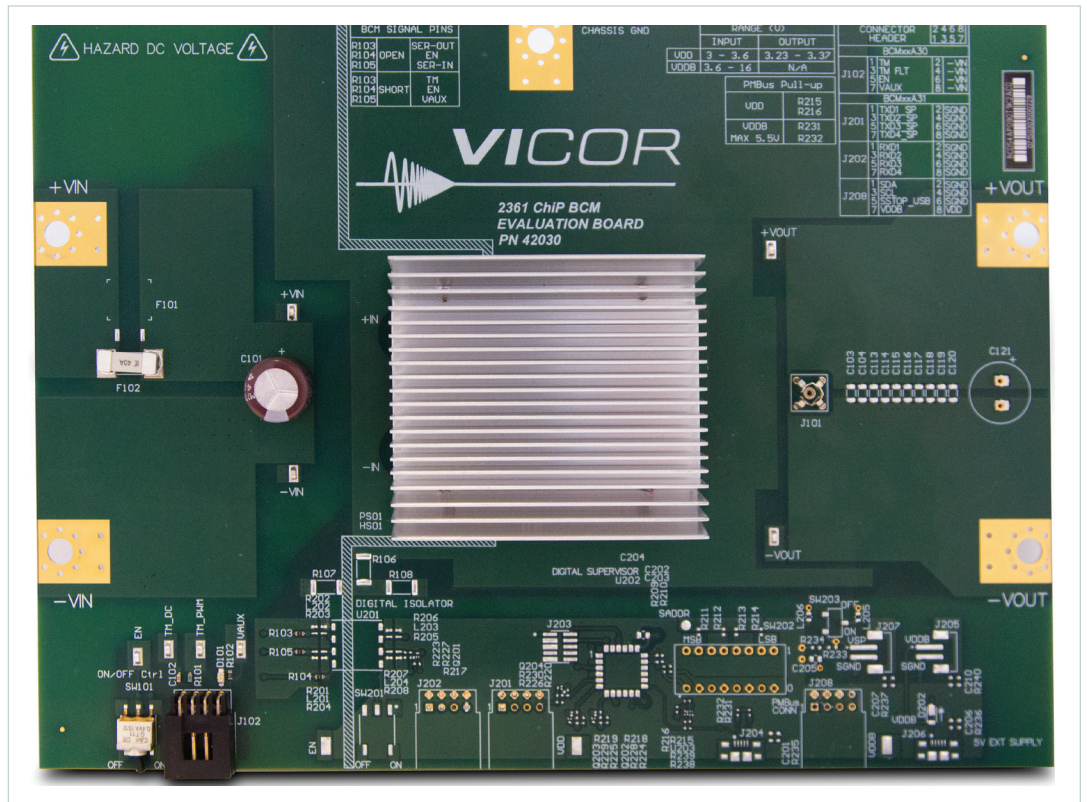
Figure 2. PCB#42030 evaluation board photo, top side
