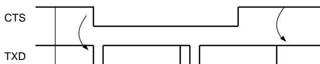
Figure 31-19. Transmitter Behavior when Operating with Hardware Handshaking
