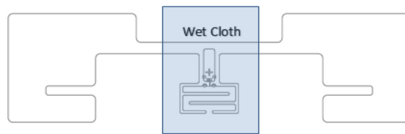
Figure 1. Moisture Contact Test Area
