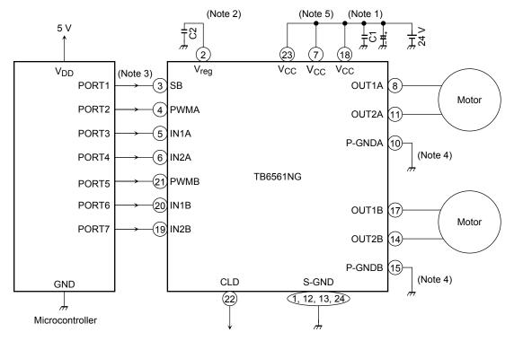
Note 1: A power supply capacitor should be connected between V<sub>CC</sub> and P-GND as close as possible to the IC.
