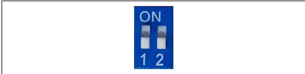
FIGURE 3-1: SW9 IN FLASH APPLICATION MODE
