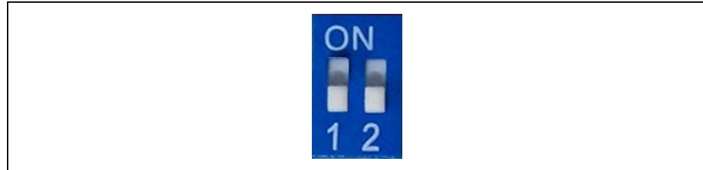
FIGURE 3-1: SW9 IN FLASH APPLICATION MODE
