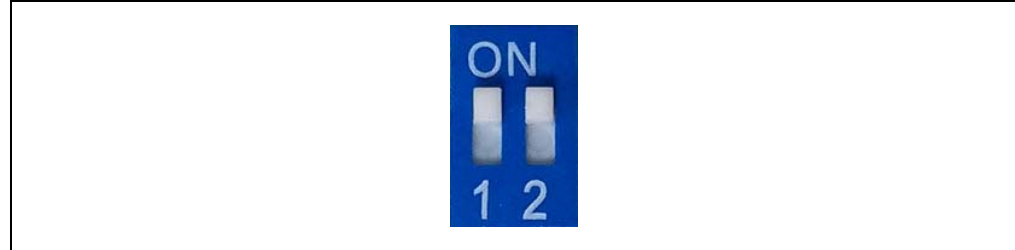
FIGURE 3-36: SWITCH SW9 IN ROM TEST MODE
