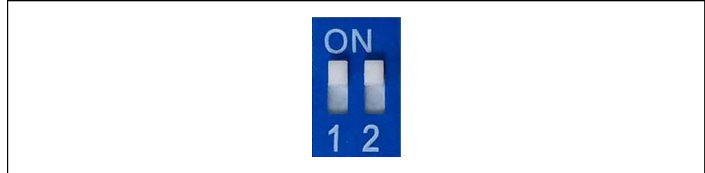
FIGURE 3-36: SWITCH SW9 IN ROM TEST MODE
