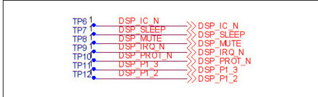
FIGURE A-11: DSP/MCU INTERFACE
