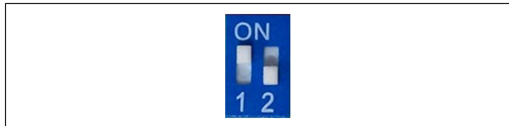
FIGURE 3-29: SWITCH SW9 IN FLASH TEST MODE
