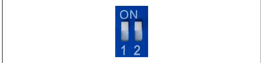
FIGURE 3-36: SWITCH SW9 IN ROM TEST MODE
