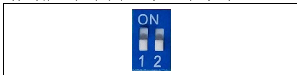
FIGURE 3-35: SWITCH SW9 IN FLASH APPLICATION MODE
