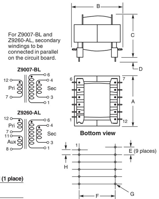
For Z9007-BL and Z9260-AL, secondary windings to be connected in parallel on the circuit board.
