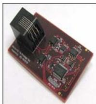
The Standard Probe Driver uses a MPLAB ICD 2 type connector (RJ-11) to connect to the target application. Designs that are compatible with MPLAB ICD 2 debugging/programming are quickly converted to use MPLAB REAL ICE. This driver board is included in the MPLAB REAL ICE In-Circuit Emulator Probe Kit (DV244005).
