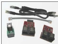
The optional Performance Pak consists of two circuit boards (driver and receiver) that employ two CAT5 cables. Debug pins are driven using LVDS communications, and additional trace connections allow high-speed serial trace uploads to the PC.
