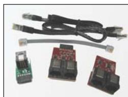
The optional Performance Pak consists of two circuit boards (driver and receiver) that employ two CAT5 cables. Debug pins are driven using LVDS communications, and additional trace connections allow high-speed serial trace uploads to the PC.
