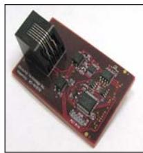
The Standard Probe Driver uses a MPLAB ICD 2 type connector (RJ-11) to connect to the target application. Designs that are compatible with MPLAB ICD 2 debugging/programming are quickly converted to use MPLAB REAL ICE. This driver board is included in the MPLAB REAL ICE In-Circuit Emulator Probe Kit (DV244005).
