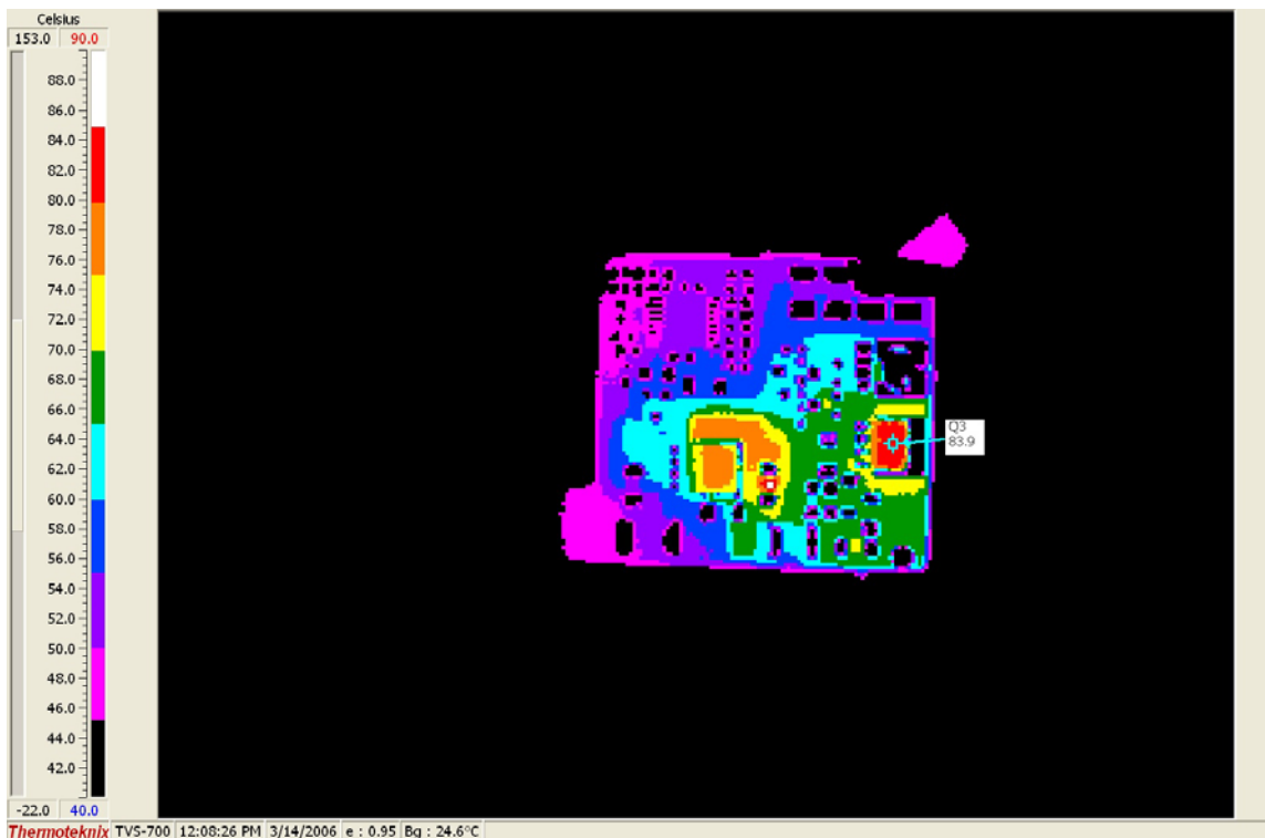
Figure 8. Temp Data (48Vin, 8A, 100LFM airflow – back)
