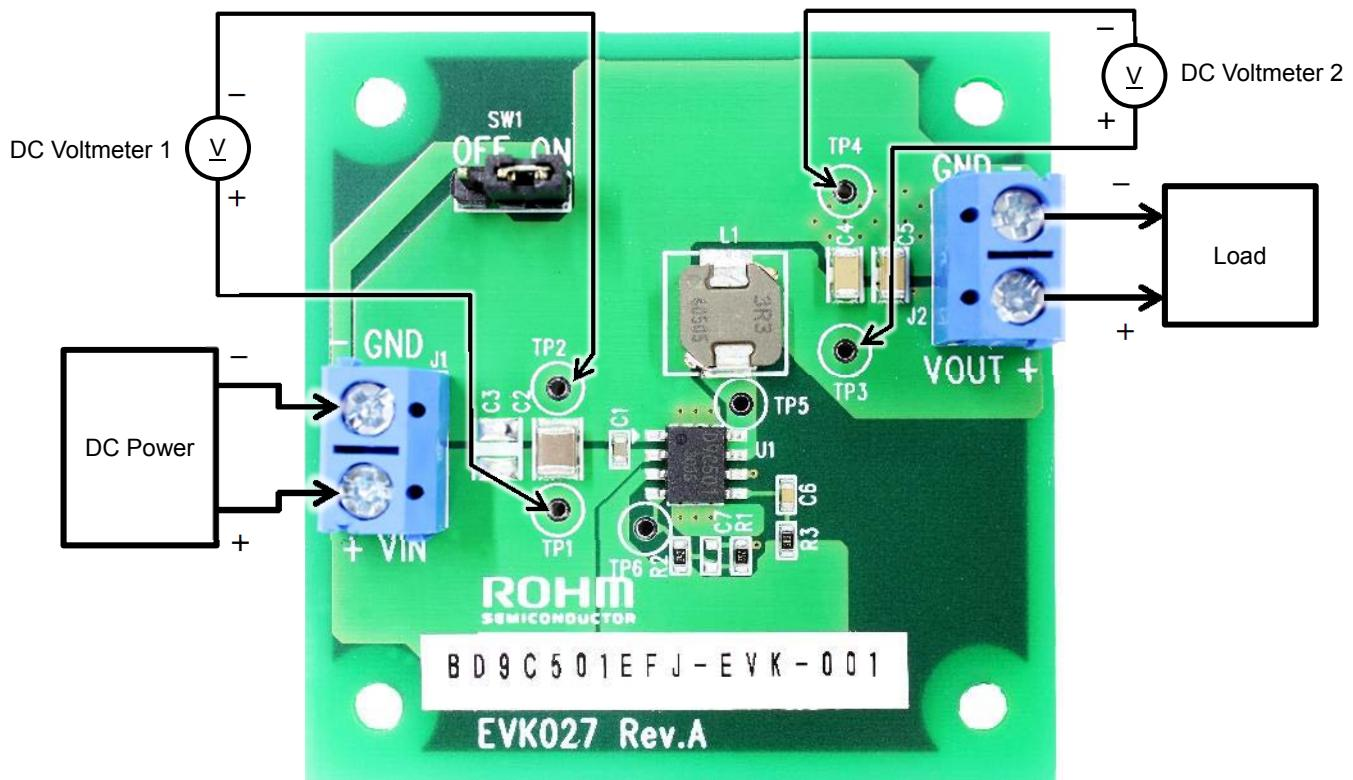
Figure 2. Connection Diagram
