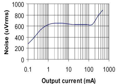
Fig. 20: Output Noise,  $C_{BYP} = \text{open}$
