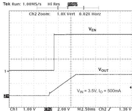
Fig. 10: Start Up Waveform,  $V_{IN}=3.5V$ ,  $I_o=500mA$
