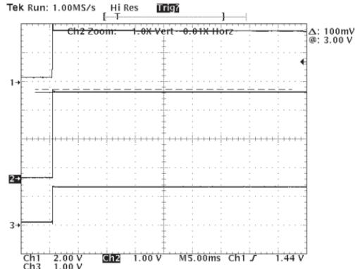
Fig. 16: Fast  $V_{IN}$ , 500mA Output Load
