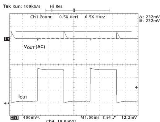
Fig. 8: Load Regulation,  $I_O=100\mu A \sim 500mA$
