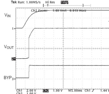
Fig. 11: Start Up Waveform, Slow  $V_{IN}$ , No Load
