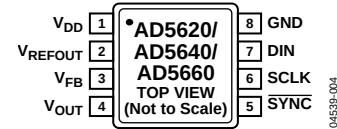
Figure 4. MSOP Pin Configuration
