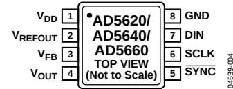
Figure 4. MSOP Pin Configuration
