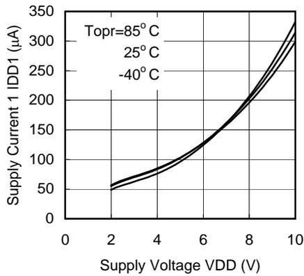
(8) Supply Current 1-1 vs. Supply Voltage
