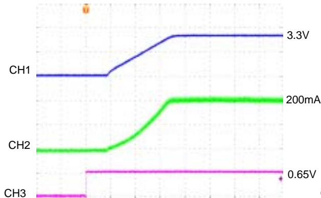
4ms/div CH1:Vout2 , 2.0V/div CH2:Iin2, 100mA/div CH3:EN2 , 0.5V/div
