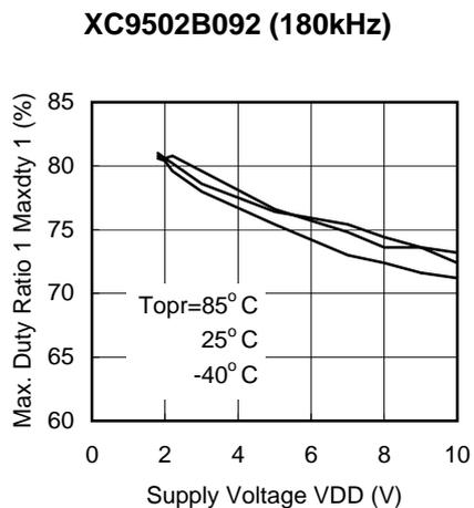
(18) PFM Duty Ratio 1, 2 vs. Supply Voltage
