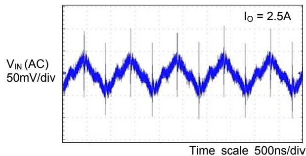
Figure 15. Input Voltage Ripple Wave
