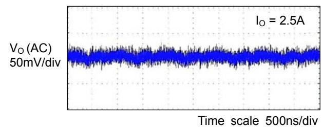
Figure 18. Output Voltage Ripple Wave
