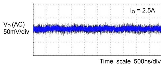
Figure 17. Output Voltage Ripple Wave
