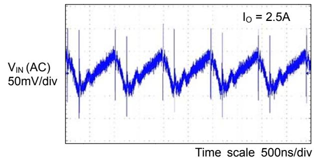
Figure 16. Input Voltage Ripple Wave
