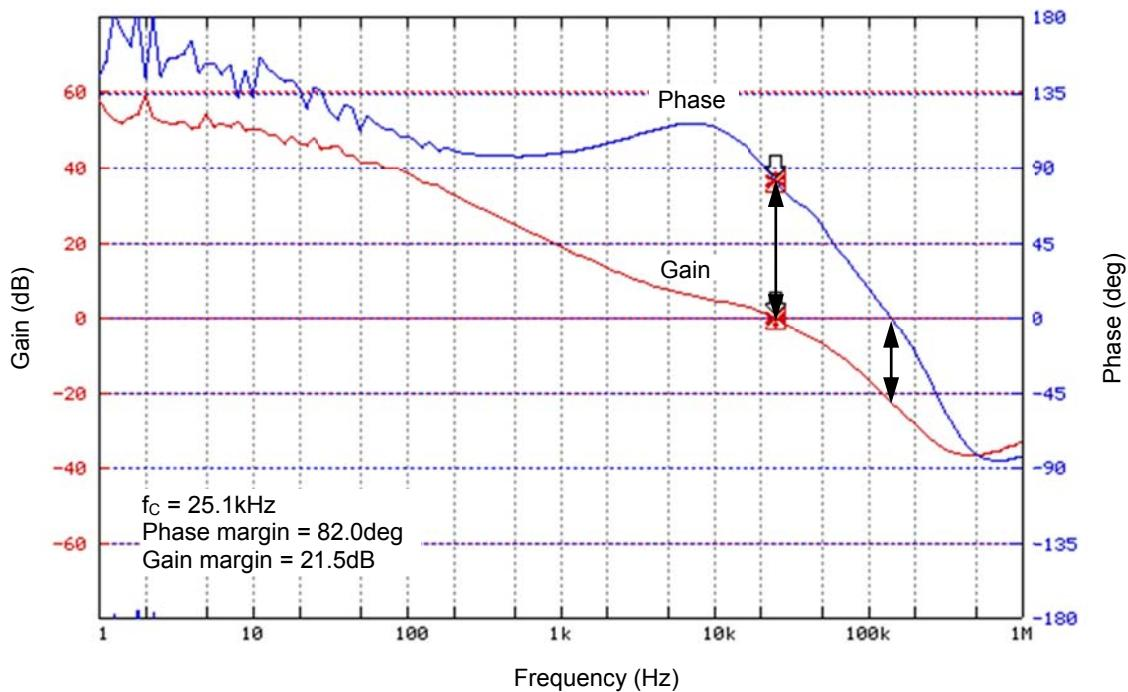
Figure 13. Loop Response  $V_{IN} = 12V$ ,  $V_O = 5.0V$ ,  $I_O = 2.5A$
