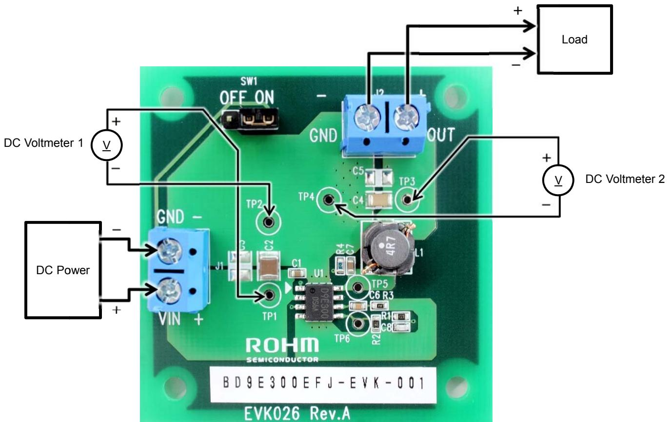
Figure 1. Connection Diagram
