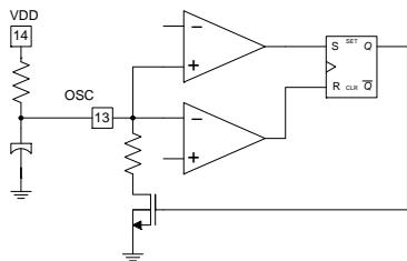
**Figure 2. Block Diagram of System Oscillator Circuit**
