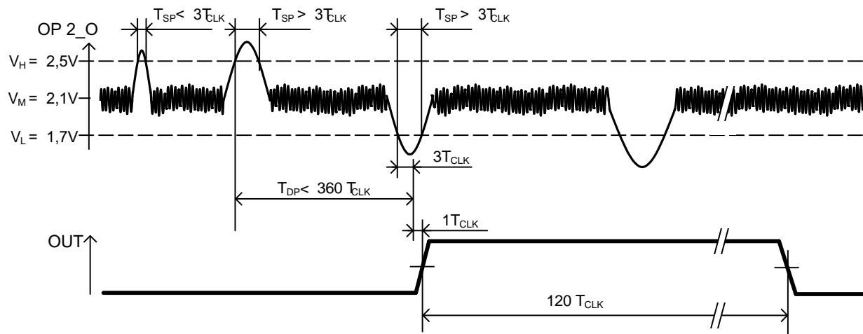
Figure 7. Timing Diagram for Dual-Pulse Mode Detection
