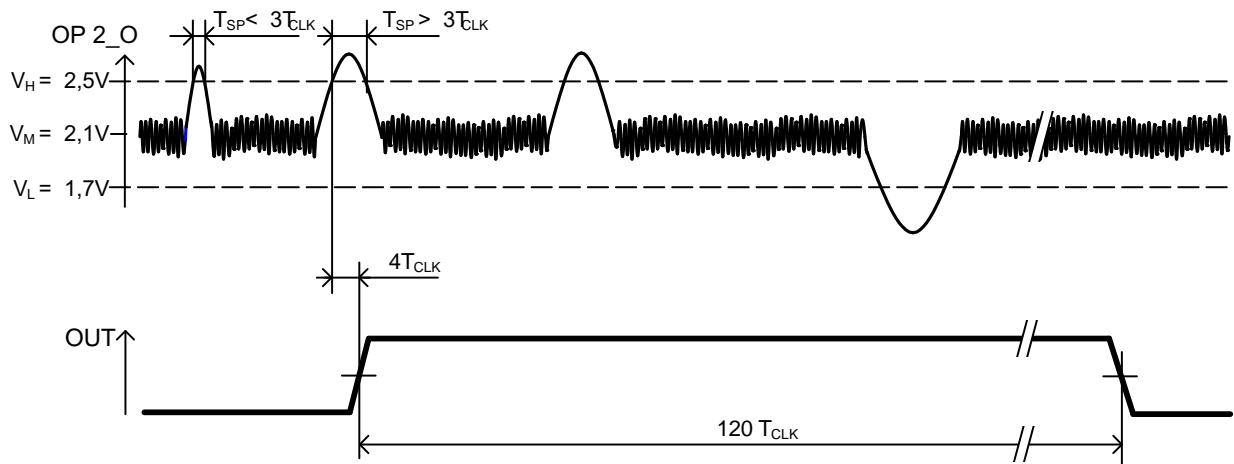
**Figure 6. Timing Diagram for Single-Pulse Mode Detection**
