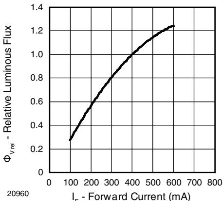
Figure 1. Relative Luminous Flux vs. Forward Current
