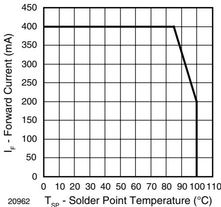
Figure 3. Forward Current vs. Solder Point Temperature
