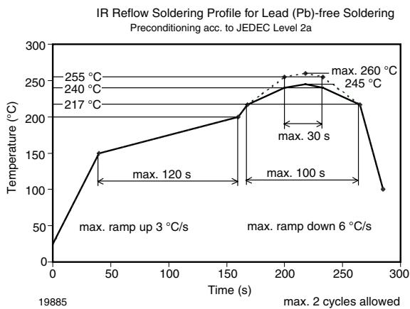
Figure 6. Vishay Lead (Pb)-free Reflow Soldering Profile
