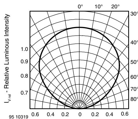
Figure 5. Relative Luminous Intensity vs. Angular Displacement
