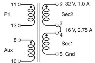
Secondary windings to be connected in series on the PC board.
