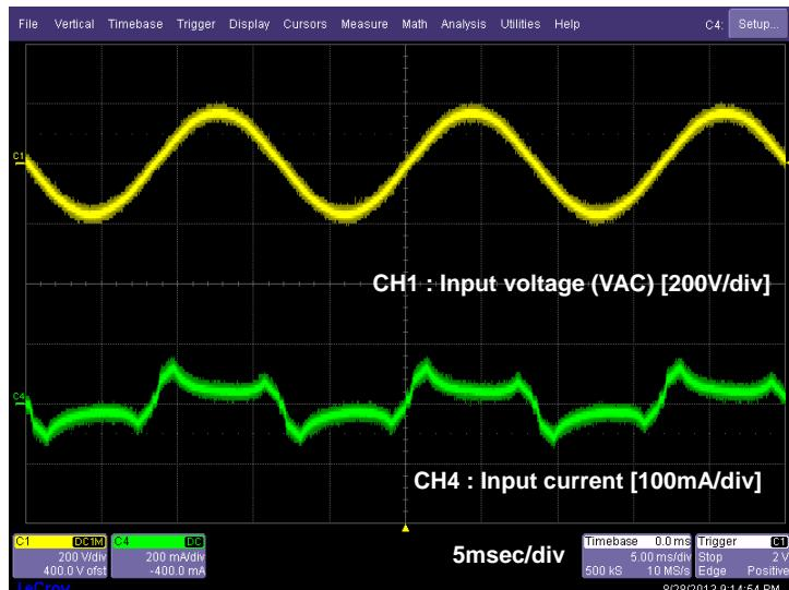
**Figure6.** Input waveform
