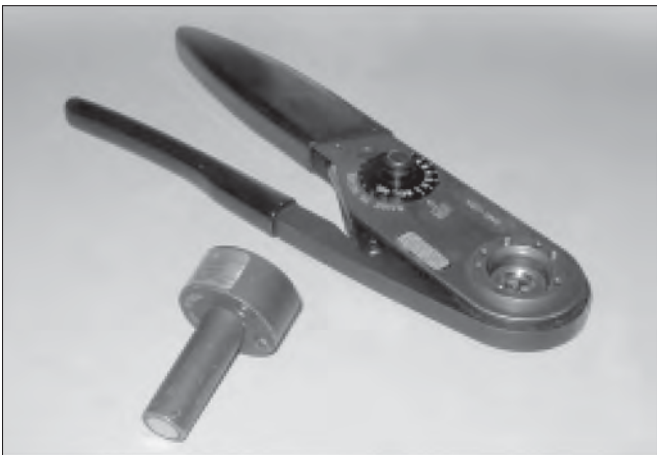
Crimp tooling M317 and locator VGE1 0078A
