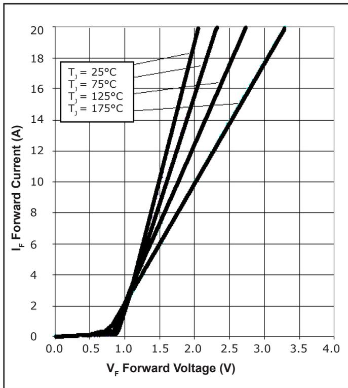
Figure 1. Forward Characteristics
