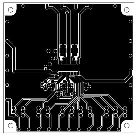
L1: Copper wiring pattern diagram
