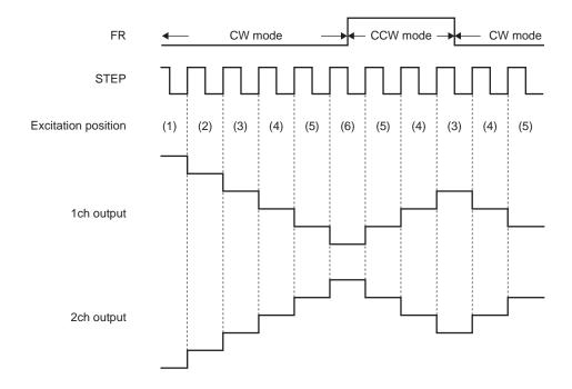
The internal D/A converter proceeds by one bit at the rising edge of the input STEP pulse.
