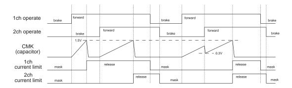
When the capacitor is not connected, the function of LIMIT in the current can be switched to operation/nonoperating state by the state of the input of the CMK pin.
