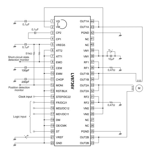
The formulae for setting the constants in the examples of the application circuits above are as follows: Constant current (100%) setting
