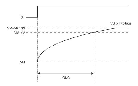
VG Pin Voltage Schematic View
