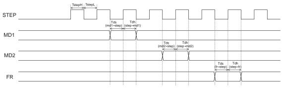
TstepH/TstepL: Clock H/L pulse width (min 500ns)
