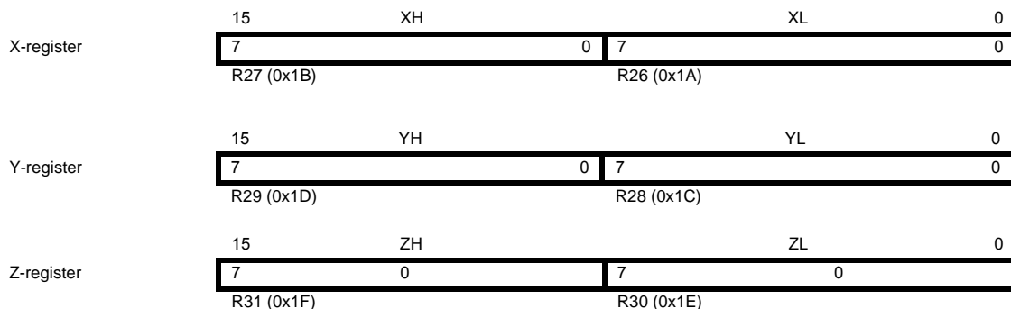
Figure 6-5. The X-, Y-, and Z-registers
