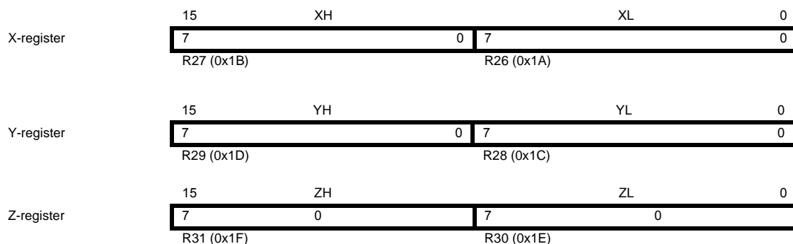
Figure 6-5. The X-, Y-, and Z-registers
