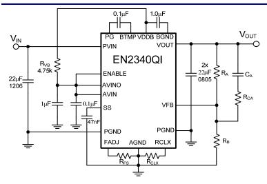
Figure 1. Simplified Applications Circuit (Footprint Optimized)
