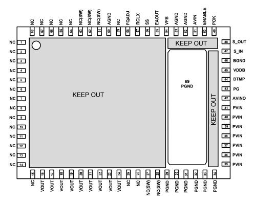
Figure 3: Pin Out Diagram (Top View)
