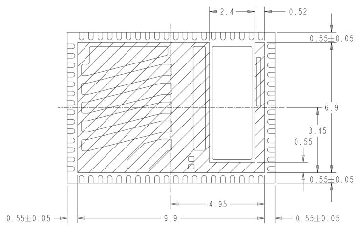
Figure 10: Lead-Frame exposed metal (Bottom View)
