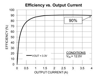
Figure 7: Efficiency vs. Output Current
