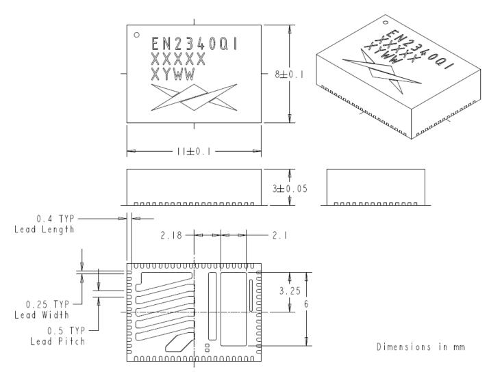
Figure 12: EN2340QI Package Dimensions (Bottom View)
