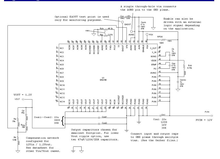
Figure 8: Engineering Schematic with Engineering Notes
