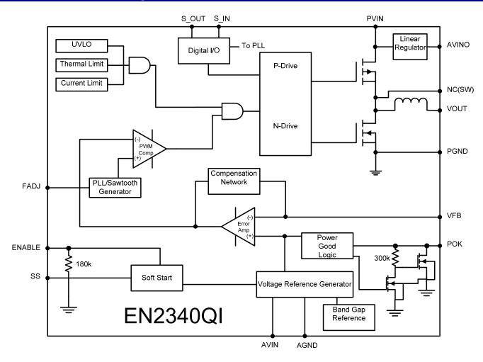
Figure 4: Functional Block Diagram
