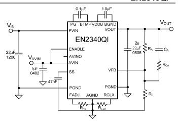
Figure 5: Dual Input Supply (PVIN and AVIN)
