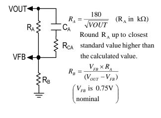
**Figure 6:** V<sub>OUT</sub> Resistor Divider & Compensation Components. RA equation is only valid for Low V<sub>OUT</sub> ripple option. For small solution size, see Table 5.
