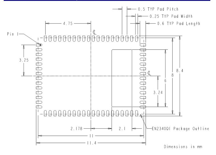
Figure 11: EN2340QI PCB Footprint (Top View)
