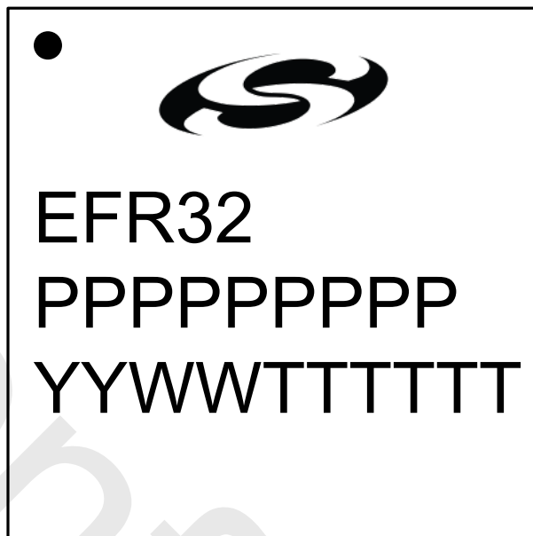
Figure 8.3. QFN32 Package Marking
