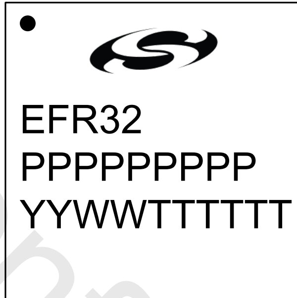
Figure 8.3. QFN32 Package Marking
