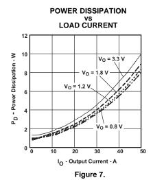
(3) The electrical characteristic data has been developed from actual products tested at 25°C. This data is considered typical for the converter. Applies to Figure 6, and Figure 7.
