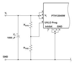
Figure 9. UVLO Program Resistor Placement
