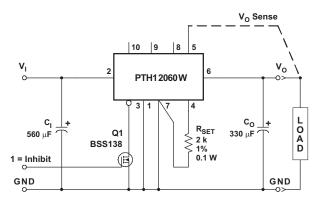
Figure 12. Inhibit Control Circuit
