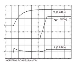
Figure 11. Power-Up Waveforms
