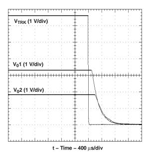
Figure 16. Simultaneous Power Down With Auto-Track Control
