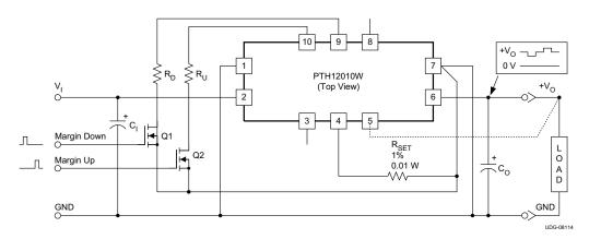
Figure 17. Margin Up/Down Application Schematic
