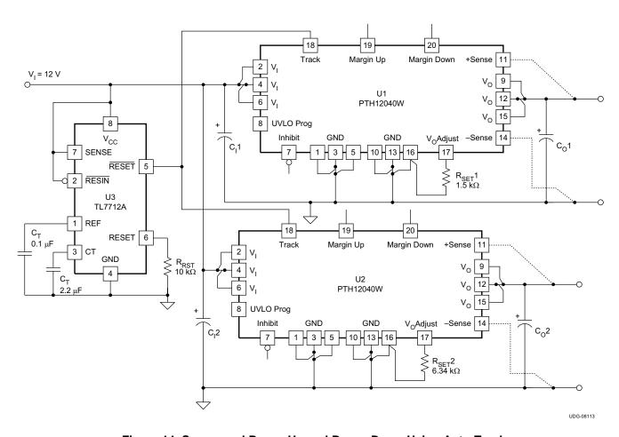
Figure 14. Sequenced Power Up and Power Down Using Auto-Track
