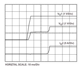
Figure 19. Pre-Bias Startup Waveforms
