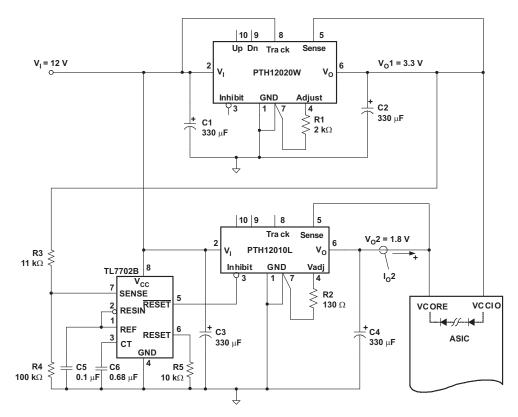
Figure 20. Application Circuit Demonstrating Prebias Startup
