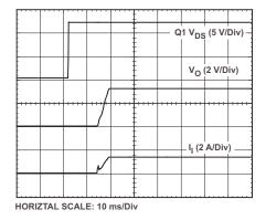
Figure 13. Power-Up from Inhibit Control
