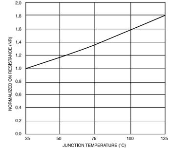
**NORMALIZED ON RESISTANCE VS JUNCTION TEMPERATURE**
