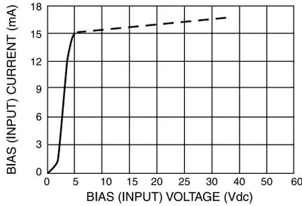
**BIAS (INPUT) CURRENT VS BIAS (OUTPUT) VOLTAGE**
