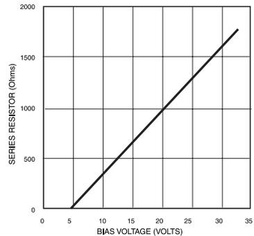
**SERIES LIMIT BIAS RESISTOR VS BIAS VOLTAGE**
