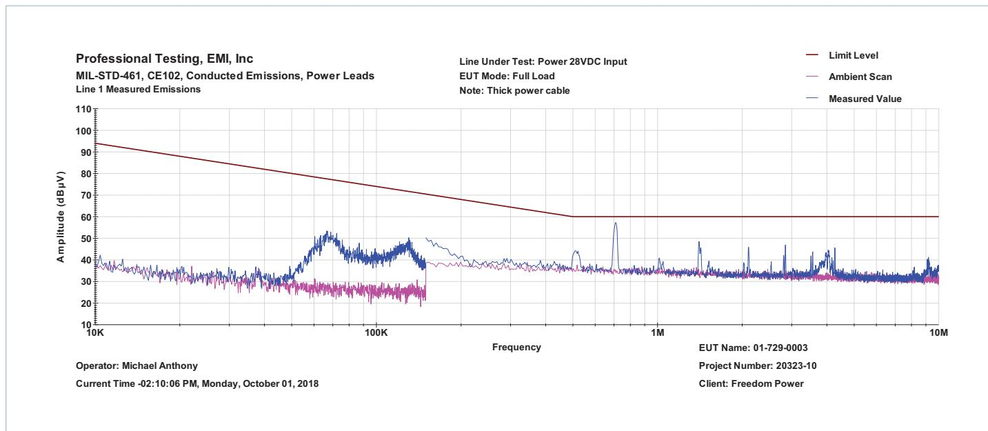
**Figure 29** — Conducted emissions of  $28V_{DC}$  input at full load
