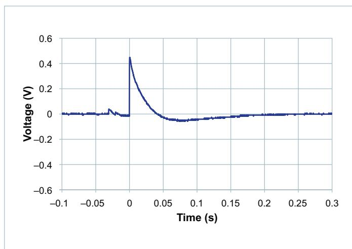
**Figure 16** — Transient response of the VS2 (+3.3V) output with a load step of 100% (20A) to 0%; AC coupled
