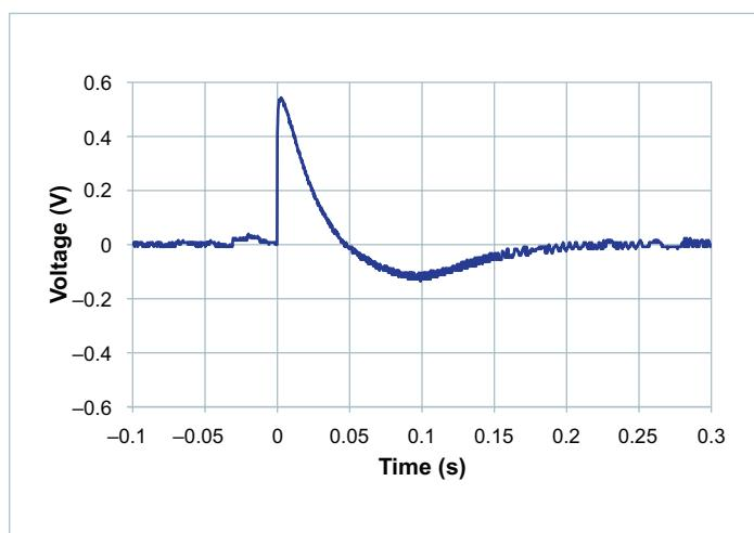
**Figure 14** — Transient response of the VS3 (+5V) output with a load step of 100% (30A) to 0%; AC coupled
